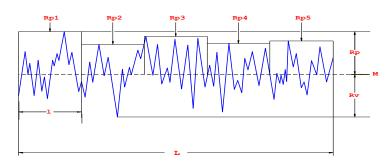
**Maximum Profile Peak Height,** *Rp*, the distance between the highest point of the profile and the mean line within the evaluation length.
