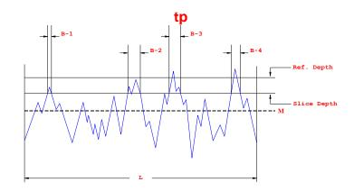
**Profile Bearing Length Ratio**, *tp*, the ratio of the profile bearing length to the evaluation length at a specified level.
