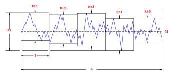
**Maximum Height of the Profile,** *Rt*, the vertical distance between the highest and lowest points of the profile within the evaluation length.
