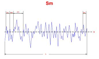
**Mean Spacing of Profile Irregularities,** *Sm***,** is the mean value of the spacing between profile irregularities within the evaluation length.
