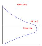
**Skewness**, *Rsk*, is a measure of the asymmetry of the profile about the mean line. A negative skewness indicates that a greater percentage of the profile is above the mean line and a positive value indicates that a greater percentage is below the mean line.
