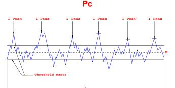
**Peak Density**, *Pc*, is the number of SAE peaks per unit length measured at a specified peak count level.
